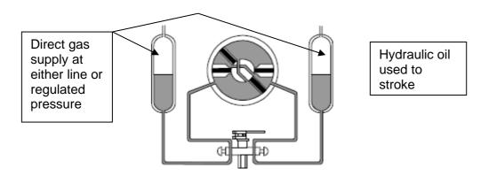
This method applies direct gas pressure onto the oil being stored in the reservoirs, therefore, forcing the oil through the actuator controls to stroke the actuator. This system will also incorporate a manual override in the form of a manual hand pump installed in the normal hydraulic circuit. Some systems have a 3rd reservoir, which is used only for the purpose of storing gas pressure in the event of a gas supply being lost.
